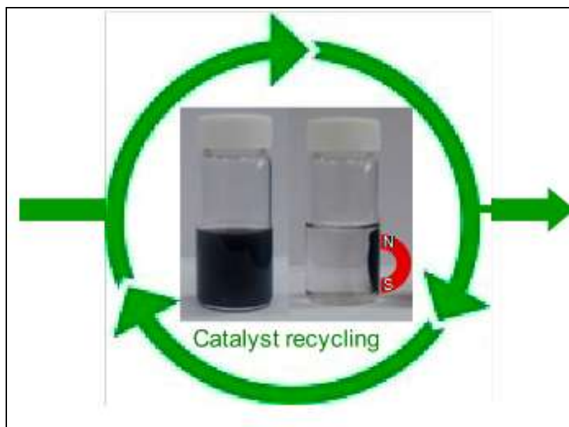
Figure 4: Separation of magnetically separable catalyst from the reaction mixture using an external magnet
