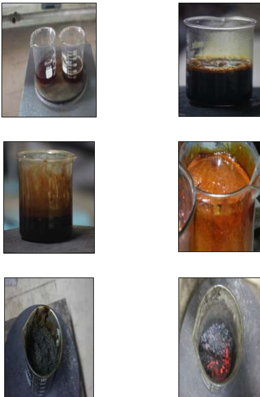
Figure 6 Synthesis of nano copper cobalt ferrites by citrate precursor method
