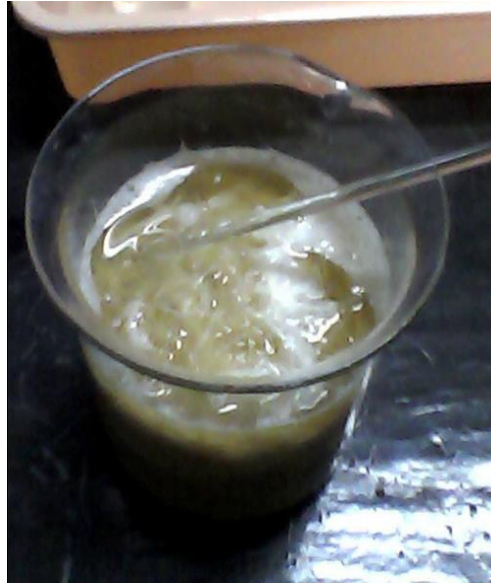
Fig.2.2 Submerged banana fibers in NaOH solution
