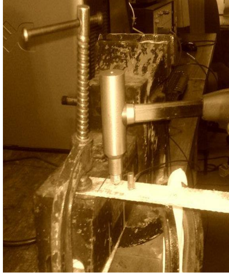
Fig.2.11 Damping test experimental set up
