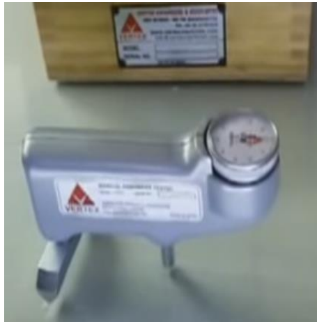
Fig.2.10 Specimens tester by barcol hardness tester
