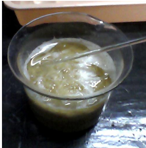
Fig.3.1 submerging banana fibers in NaOH solution.
