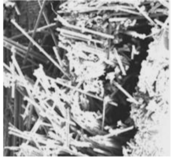
Fig.3.13SEM micrograph of fractured surface of 6wt.% banana nanofiber composite
