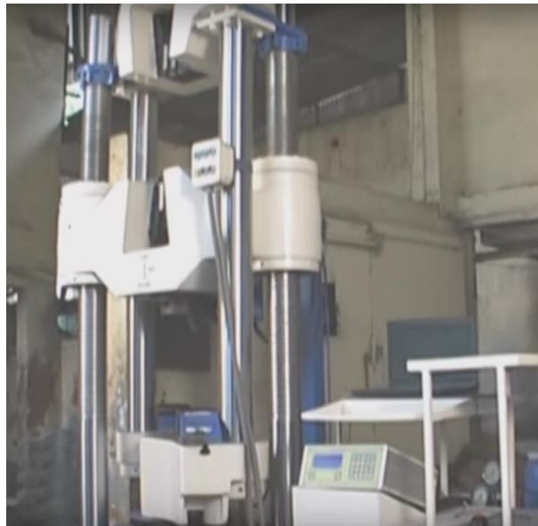
Fig.2.4 Computerized UTM (Tinus Olesan)
