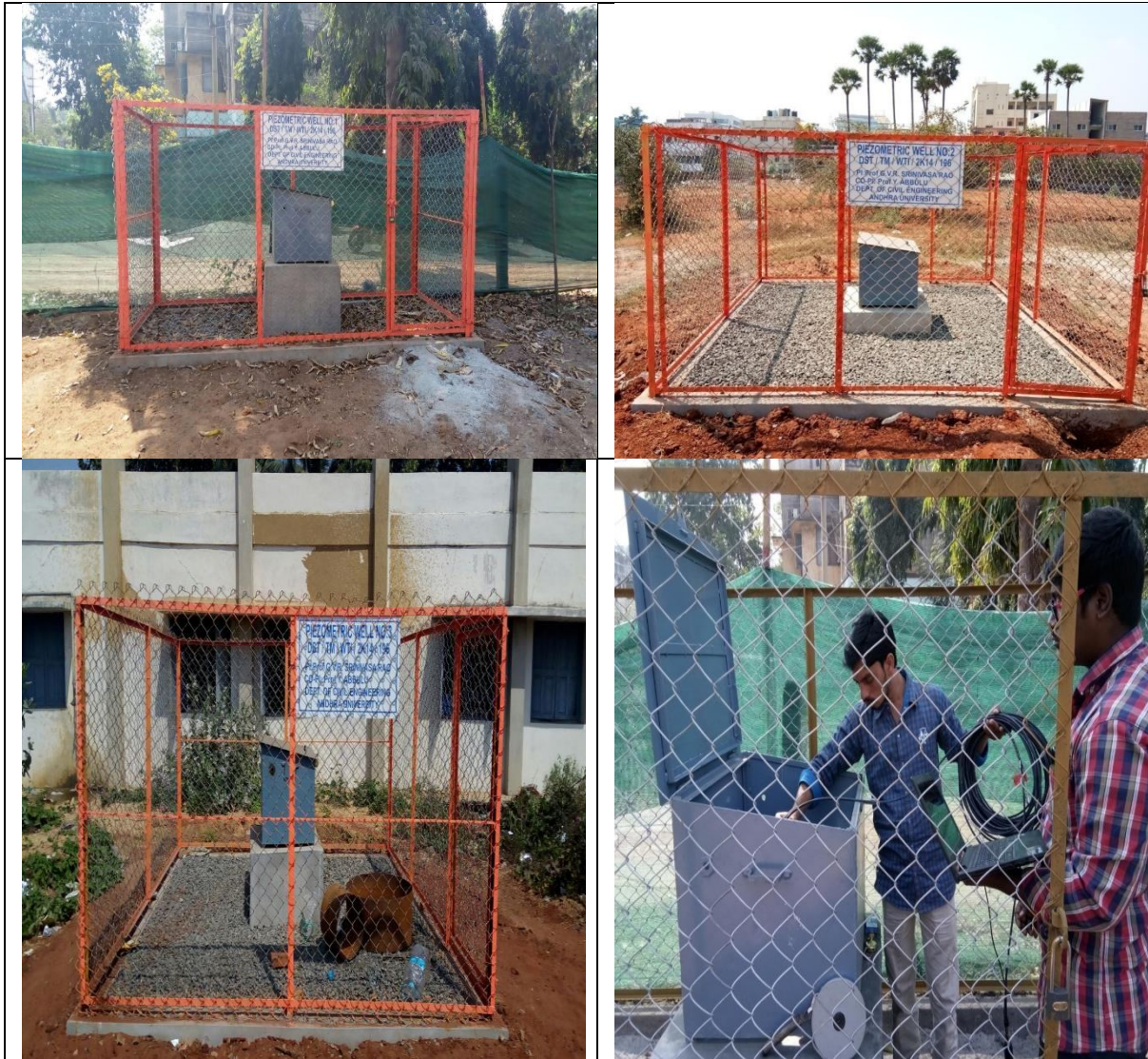
Figure 15: Typical RWH Monitoring Wells in the Andhra University Campus.
